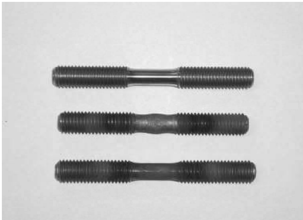
Fig. A1.2: Strain reversal test specimens subjected to compression and tension
